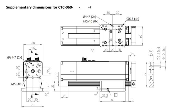
[1] Conical grease nipple for lubricating the guide (both sides)
